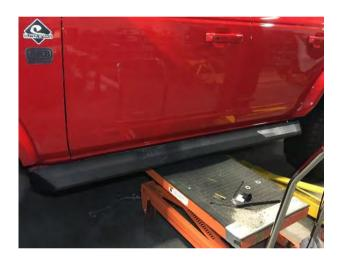
7. Using a lift table or a friend, lift the sliders into position and fasten the two body mount nuts onto the studs. Leave loose for now.
