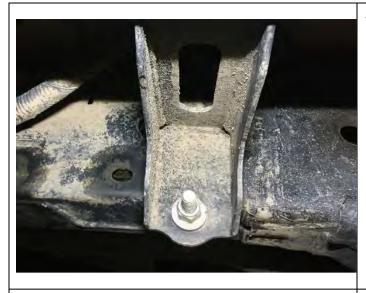
10. Using 2x M12 nuts and washers, fasten the slider to the u-bolt Leave loose for now.
