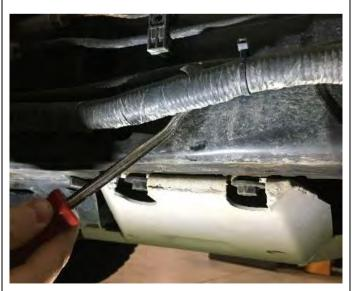
4. Using a body clip tool, loosen the wiring harness from the length of the left side frame rail. On the inboard side of the left frame rail, also disconnect the brake lines in the rear.
